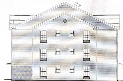
GUEST WING 'B' RIGHT BUILDING ELEVATION 1/8"=1'-0"
