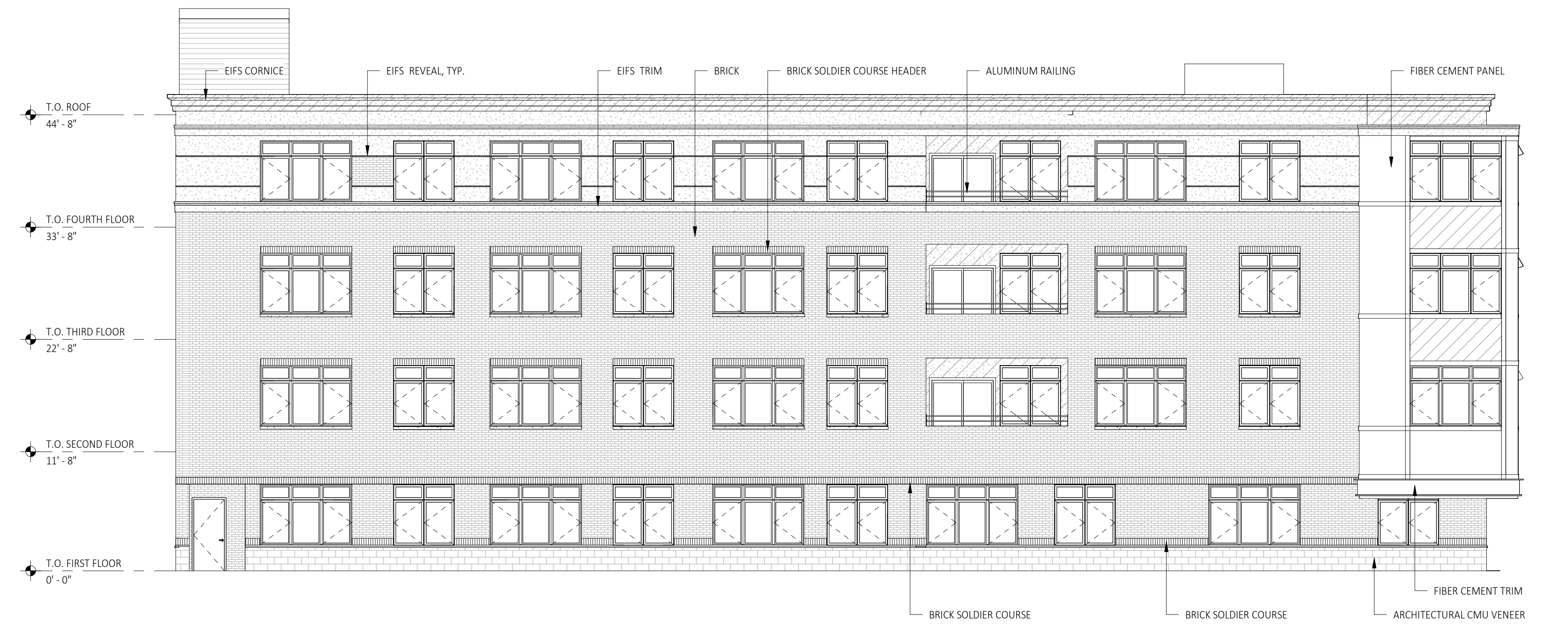
1 Building Elevation at Lark Street A200 SCALE: 1/8" = 1'-0"
