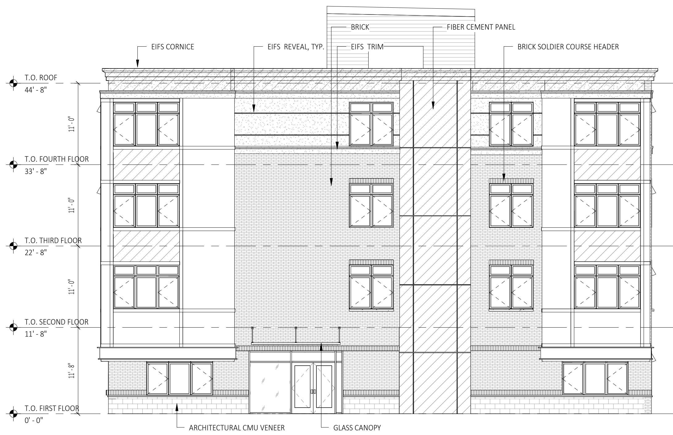
3 Building Elevation at Morris Street A200 SCALE: 1/8" = 1'-0"
