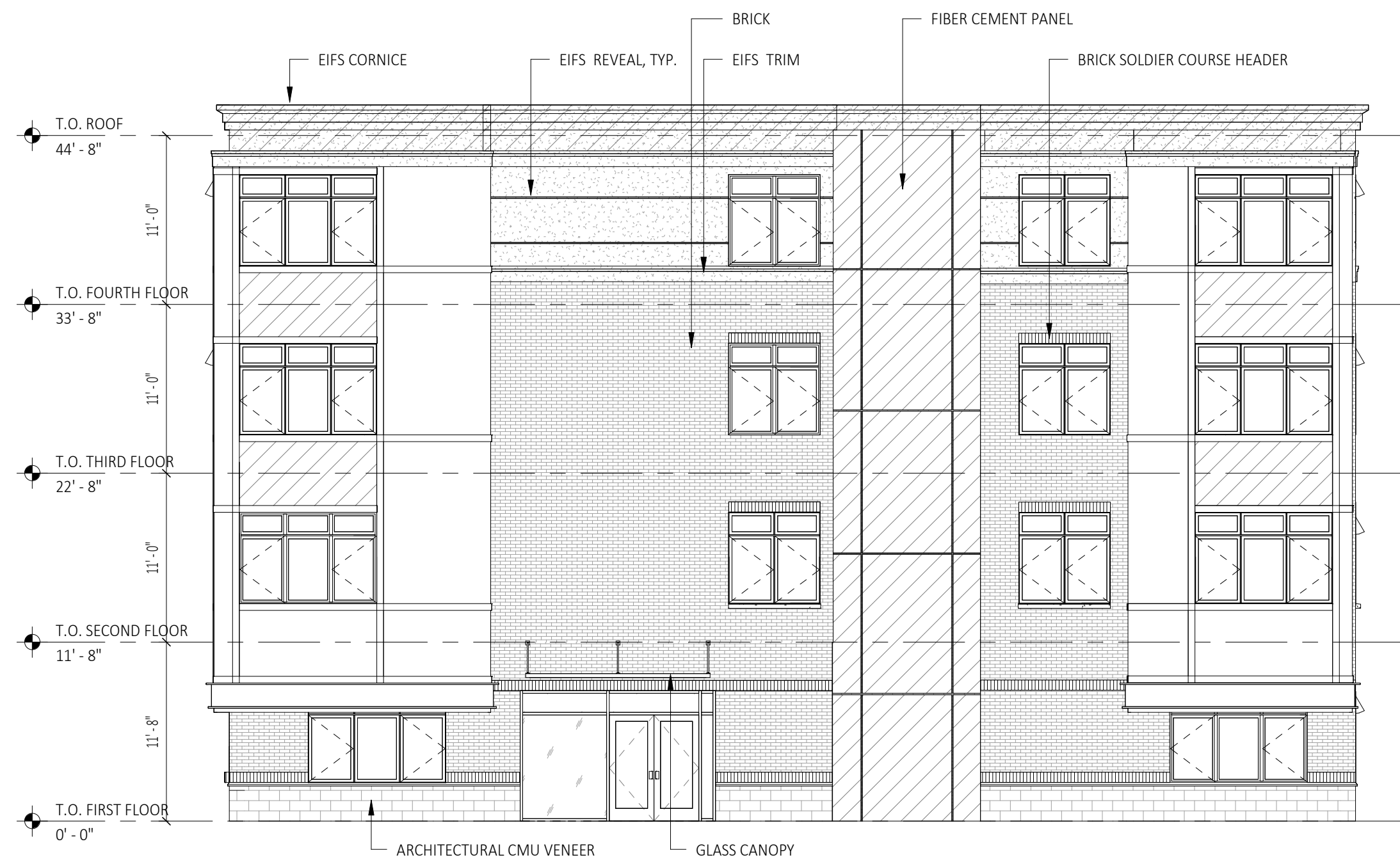
3 Building Elevation at Morris Street A200 SCALE: 1/8" = 1'-0"
