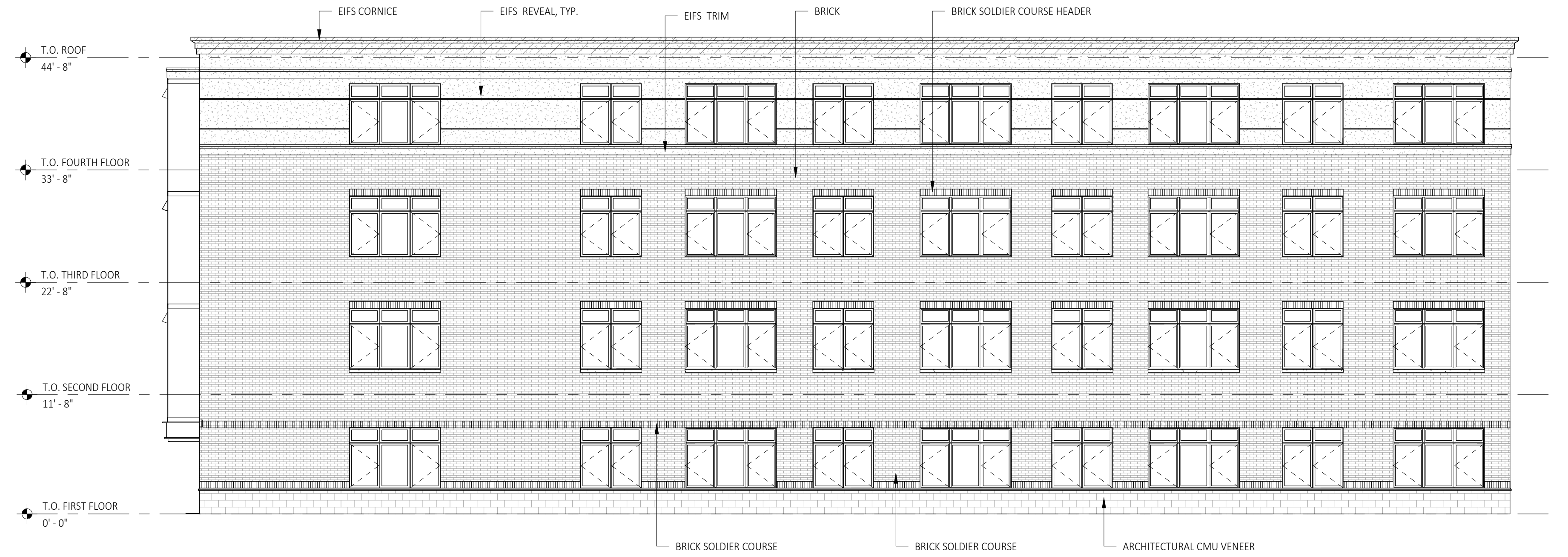
2 Building Elevation - North A200 SCALE: 1/8" = 1'-0"
