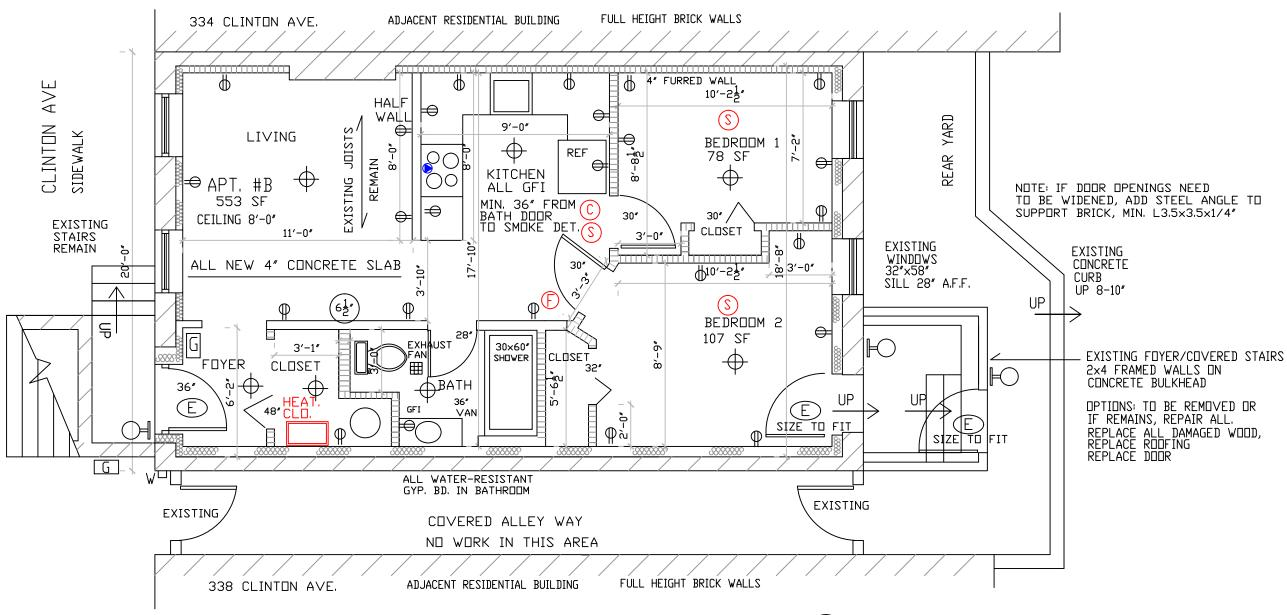
NOTE: EXHAUST FAN DUCTS TO GO THRU ROOF OR A LOCATION APPROVED BY ALBANY'S HRC.
