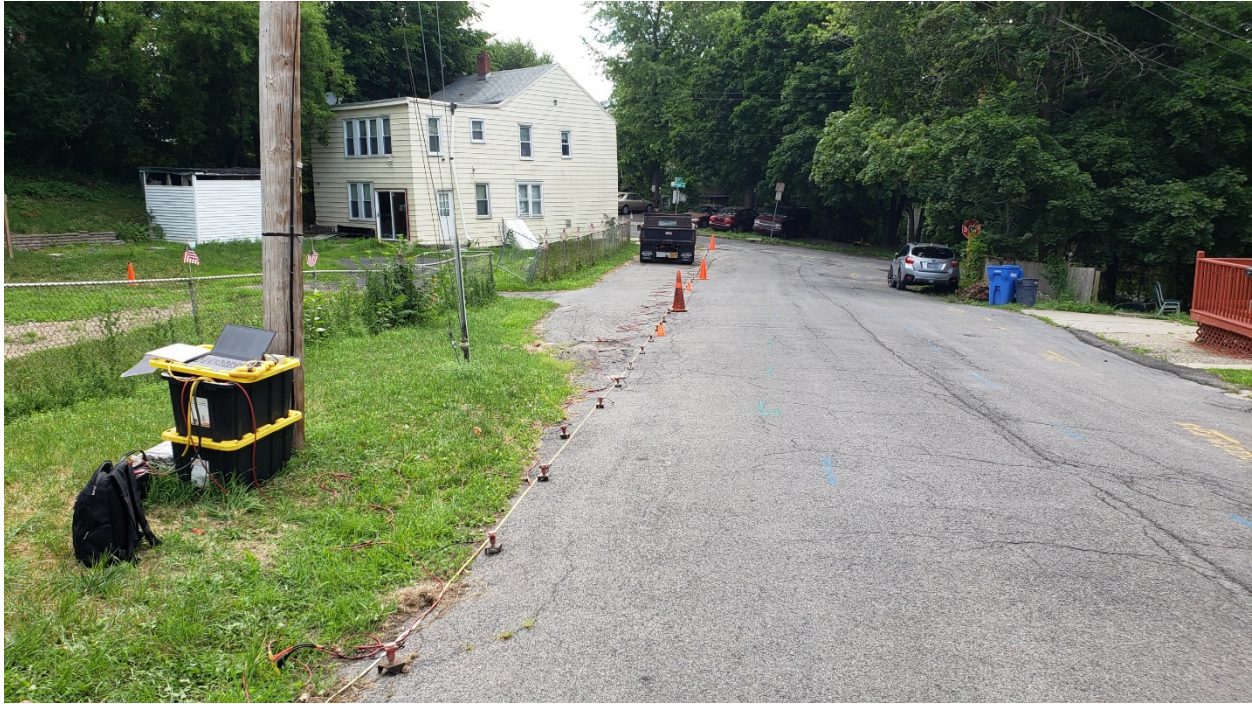
Photograph 1. Typical conditions at the site, view to the east along Scott Street. The array for Seismic Line 1 is located along the measuring tape in the center left of photograph.
