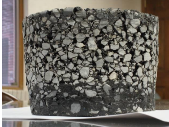
Core taken 3 days after placement with 6.5% asphalt binder . Note accmulation of asphalt binder at the bottom of core.
