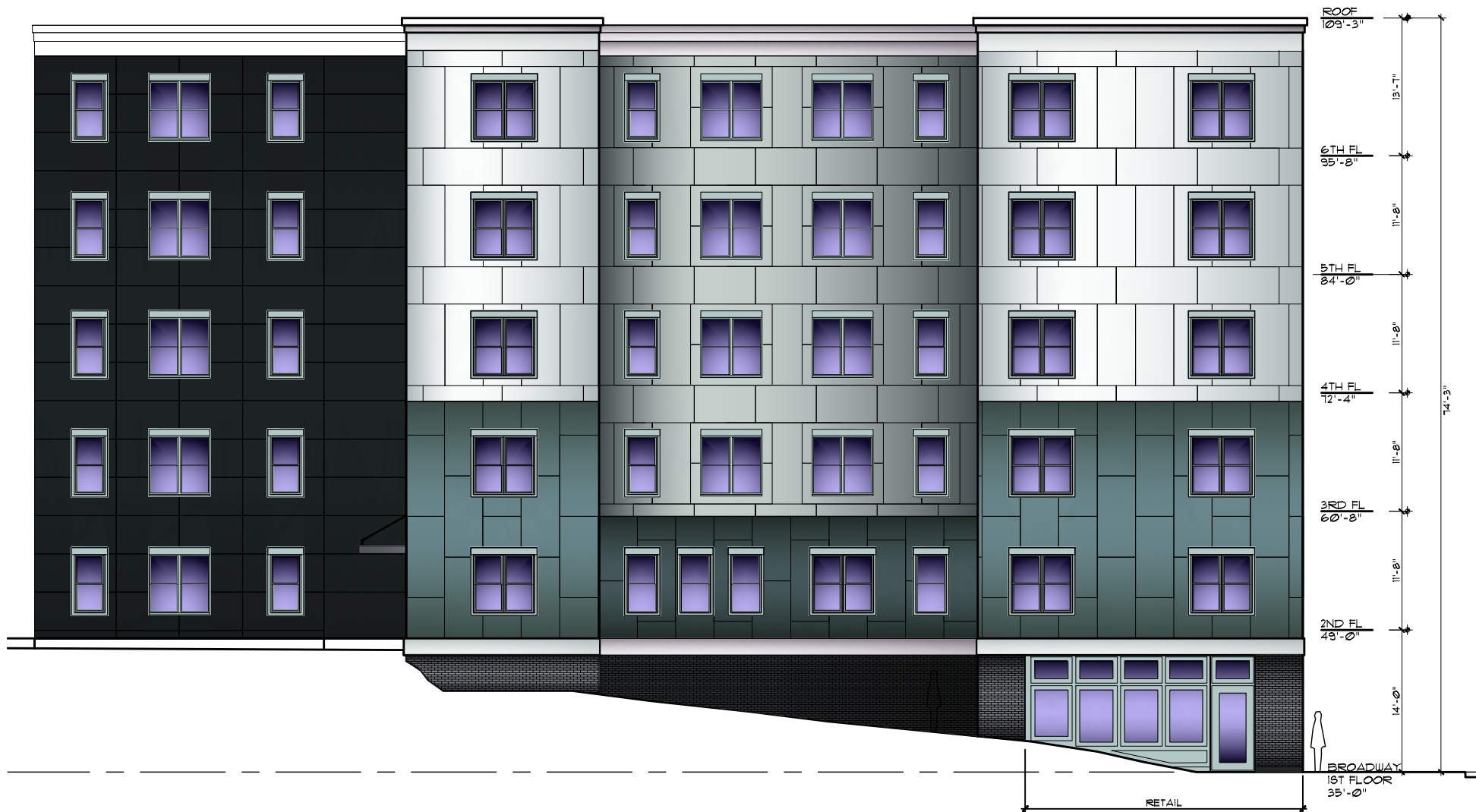
C. 1 LIGHT WINDOW TRIM / VERTICAL PANEL ORIENTATION
