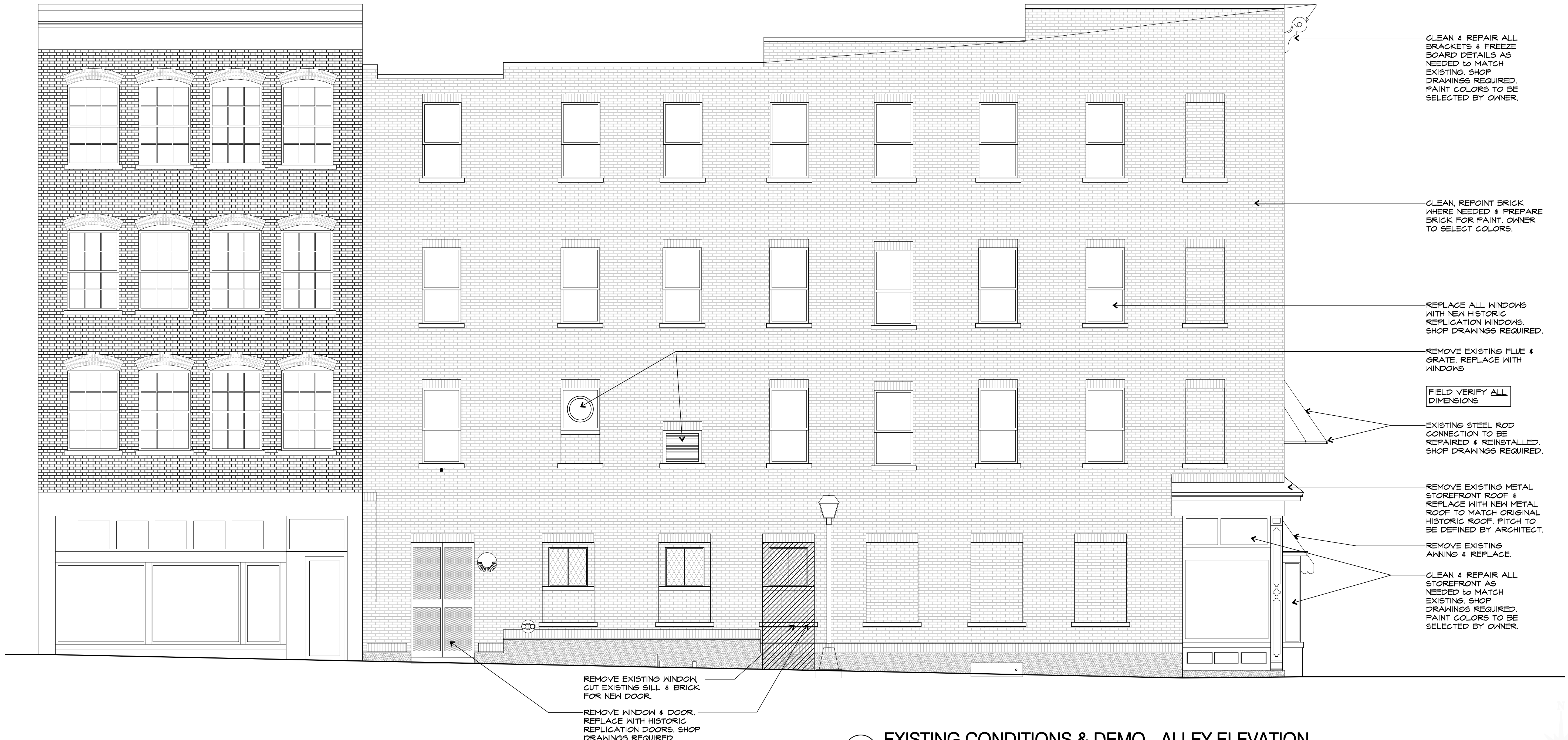
1 EXISTING CONDITIONS & DEMO - ALLEY ELEVATION SCALE: 1/4" = 1'-0"
