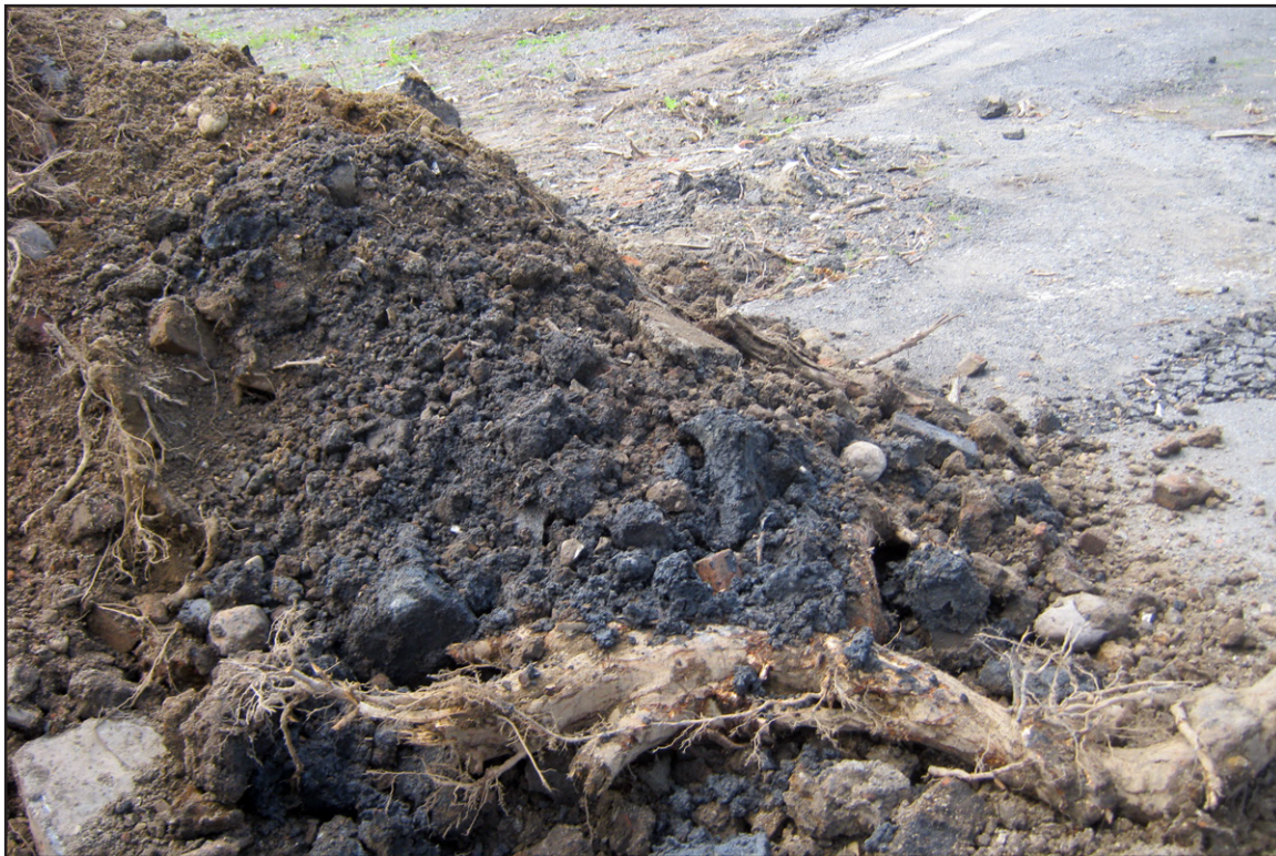
PHOTOGRAPH 4: Contaminated Material from Stratum D in Trench 1
