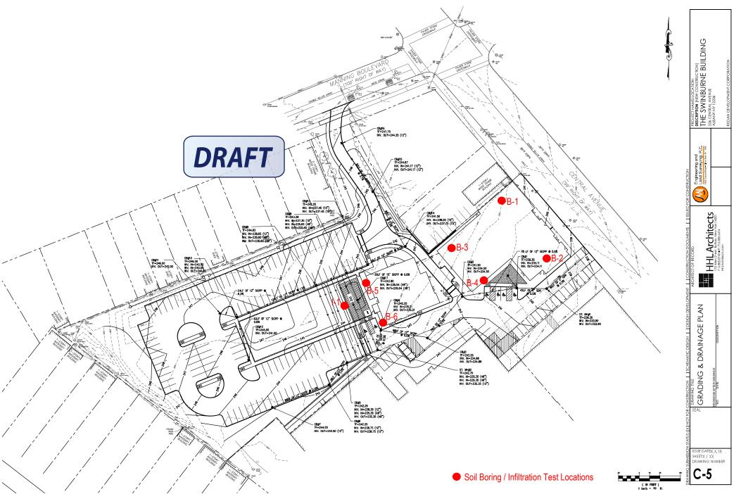
SUBSURFACE LOG: B-1 DENTE GROUP, A TERRACON COMPANY PROJECT: 526 Central Avenue DATE START: 2/22/18 FINISH: 2/22/18 **LOCATION**: Albany, New York METHODS: 3 1/4" Hollow Stem Augers, ASTM DRAFT 586 Drilling Methods with Auto Hammer FACE ELEVATION: +/- 242.0' CLIENT: Regan Development Co JOB NUMBER: JB185008 **DRILL TYPE**: CME 45C **CLASSIFICATION:** O.Burns SAMPLE **BLOWS ON SAMPLER** CLASSIFICATION / OBSERVATIONS
