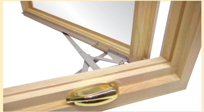
The concealed 2-bar "Washability Hinge" is tamper resistant and allows for quick and precise sash re-alignment within the window frame. The snap-ring detach feature also allows for quick sash removal. A nylon shoe slides along the stainless steel hinge track providing self cleaning action for longer life. Egress and 4-bar hinges are also available.
