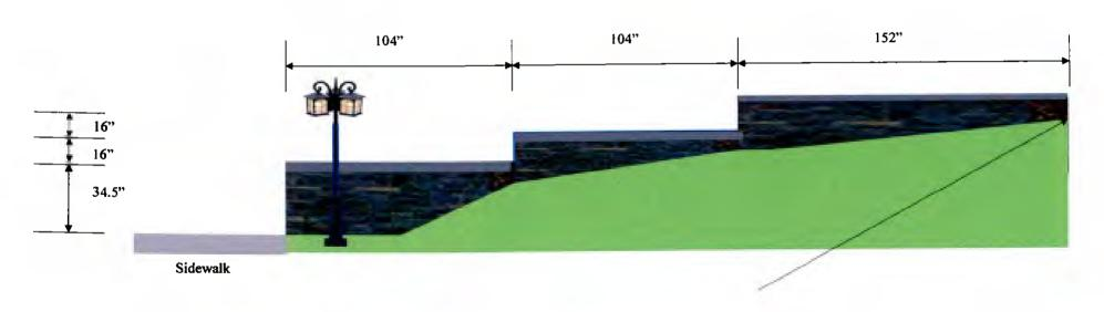
The highest level of fill on the house side of the wall is 72" higher than the sidewalk to the new basement door.
